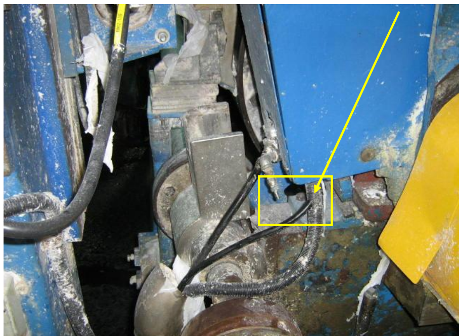
Airline to B/S cylinder (to open primary arm clamp) came off fitting
