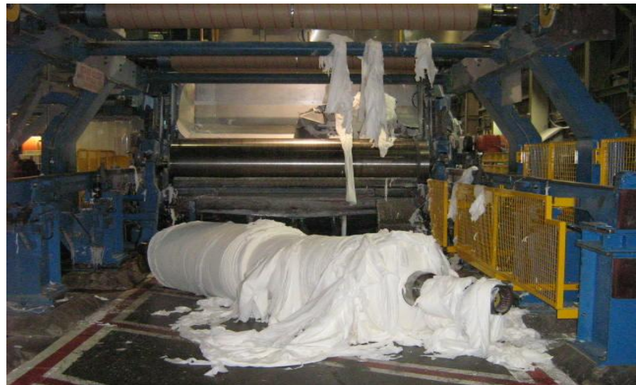
Ejected reel on floor between the rails
