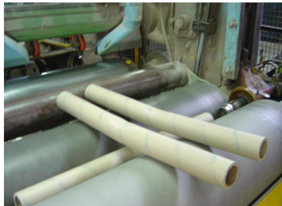
Impact of pressure on core from 'Rider' Roll
